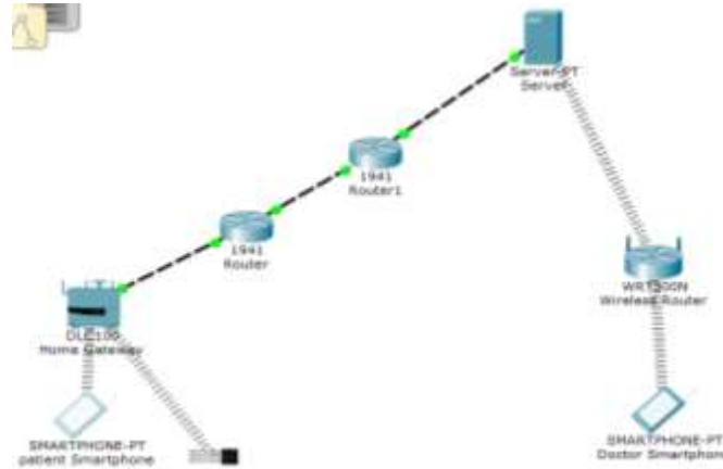
FIGURE 2. Network verification using Cisco Packet Tracer.
