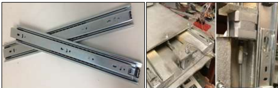
FIGURE 3. (a) Drawer Slide (left), (b) Stepper motor coupling with slide (right)
