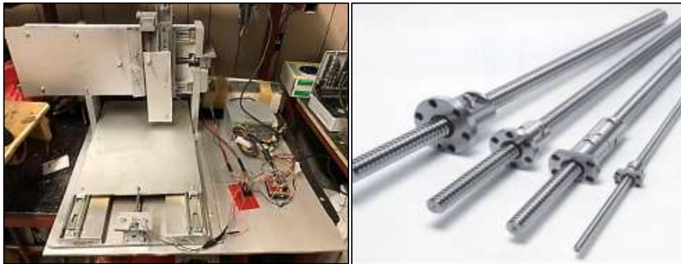
FIGURE 2. a) The CNC System (left), b) Ball Screws (right)
