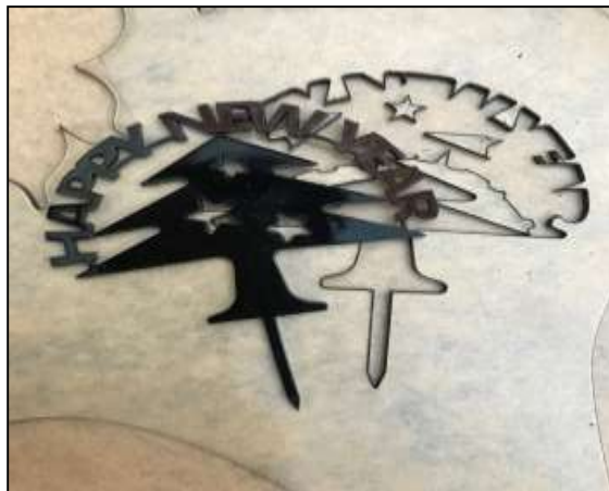
FIGURE 12. Designed shape engraved by laser on acrylic material
