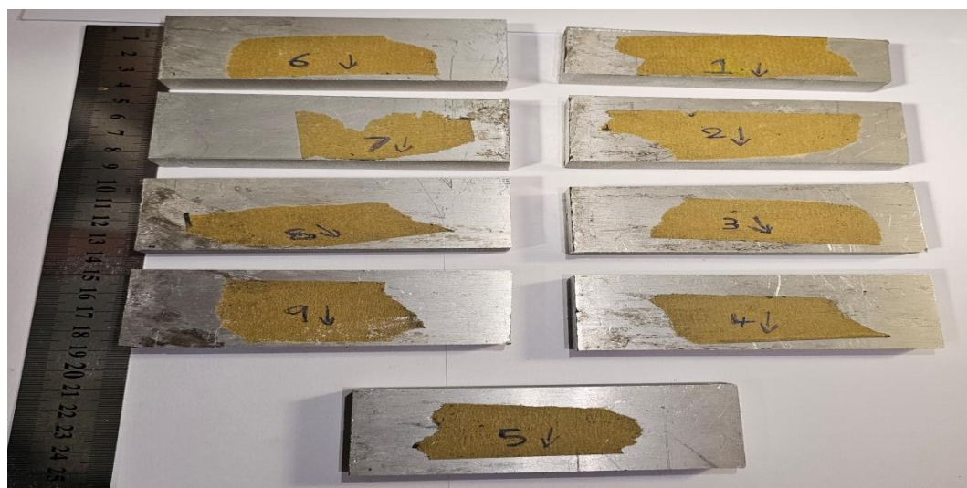
Fig.3. Machined AA6061 specimens (15 mm thick) labeled 1–9 after abrasive water jet cutting based on the Taguchi L9 design, representing different combinations of water pressure, traverse speed, and stand-off distance. Arrows indicate the cutting direction.
