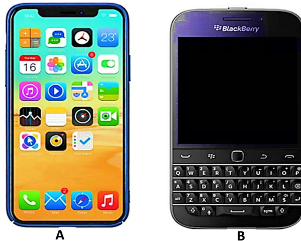
Figure (1): A) Smart Phone without physical Buttons, B) Blackberry Mobile with Physical Buttons.
